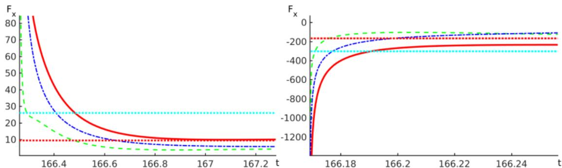
**Figure :** The structure of hydrodynamic forces in forward and backward motion zones. The red solid line indicates the total inline hydrodynamic force  $F_x$ , the cyan dotted line represents the average force per phase  $F_{av}$ , and the red dotted line represents the quasistationary approximation  $F_{st}$ .  $\kappa = 0.6$ ,  $Re_{av} = 25$ ,  $b = 0.08$ .
