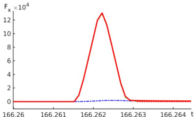
**Figure :** The structure of hydrodynamic forces in accelerated motion zone. The red solid line indicates the total in-line hydrodynamic force  $F_x$ , the blue dash-dotted line represents the component associated with the viscous stresses  $F_v$ , the green dash line represents the component associated with the pressure distribution  $F_p$ .  $\kappa = 0.6$ ,  $Re_{ov} = 25$ .
