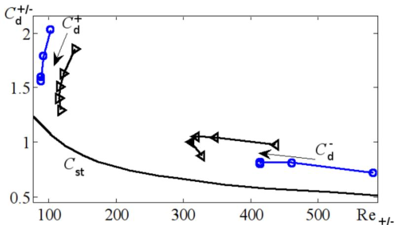
Figure : Values of  $C_d^{+/-}$  for  $Re_{av} = 47$ ,  $b = 0.16$ ,  $\kappa = [0.7015, 1.403, 2.1045, 2.806, 5.612]$  (black markers) and  $Re_{av} = 47$ ,  $b = 0.08$ ,  $\kappa = [1.09, 2.19, 4.38, 5.48]$  (blue markers). The arrows indicate the direction of growth of  $\kappa$ . The black solid line represents the values of  $C_{st}$ .
