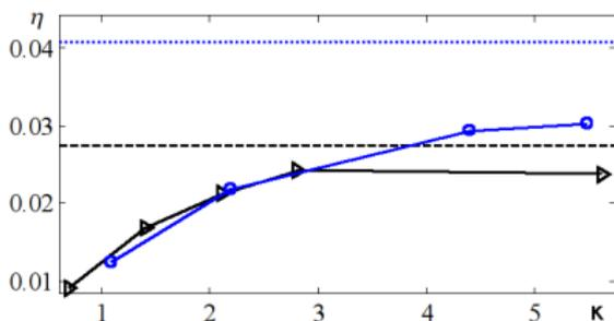
**Figure :** Efficiency of the propulsion mechanism.  $Re_{av} = 47$ ,  $b = 0.16$ ,  $\kappa = [0.7015, 1.403, 2.1045, 2.806, 5.612]$  (black markers) and  $Re_{av} = 47$ ,  $b = 0.08$ ,  $\kappa = [1.09, 2.19, 4.38, 5.48]$  (blue markers). The lines represents the estimates of theoretical efficiency.
