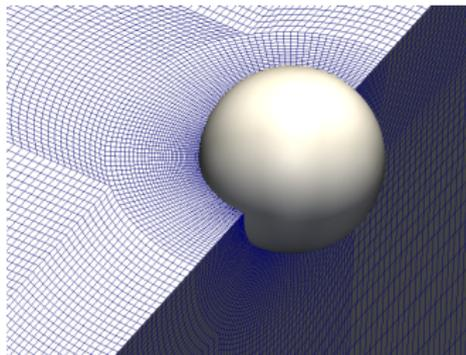
Figure : Three-dimensional mesh structure in the vicinity of the sphere.
