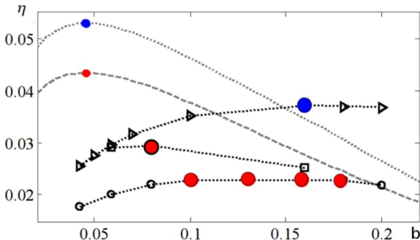
**Figure :** The efficiency of motion as a function of the phase duration. Black lines with markers represent numerical simulation data:  $KC = 2.2$ ,  $Re = 47$  (round markers),  $KC = 2.2$ ,  $Re = 102$  (triangular markers) and  $KC = 4.4$ ,  $Re = 47$  (square markers).
