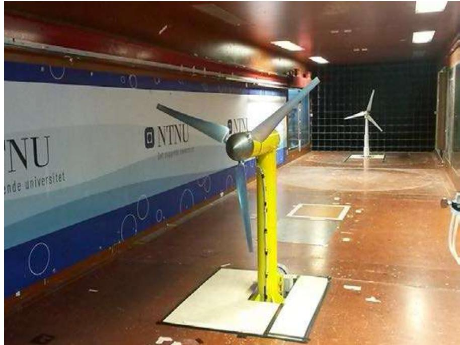
Fig. Model wind turbines in the wind tunnel ( $x/D=9.00$ ) in NTNU, Trondheim, Norway
